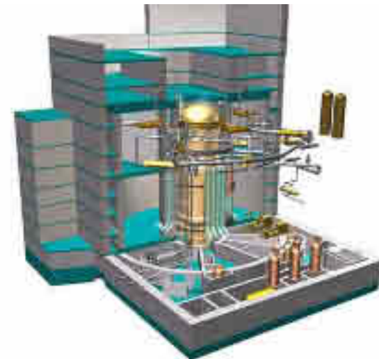
Boiling Water Reactor 1,250 MWe Passive safety
