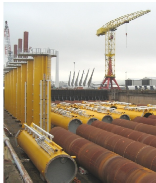
Port storage for monopiles
