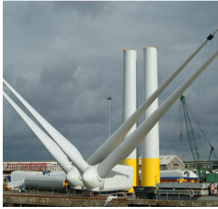
Pre-assembled turbine parts in the harbour
